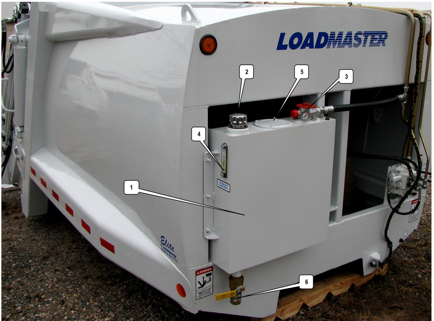
ELITE "OIL TANK" WELD ASSY
