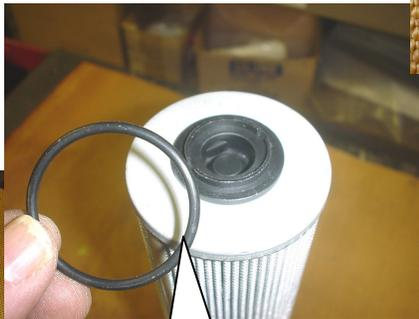
**3, the 0-ring is included with each Element and is at very Bottom of canister, between bottom of Element and Canister's inside bottom. Inspect old o-ring (with PenLite) and replace O-ring "if needed" at time of installing a fresh Element**
