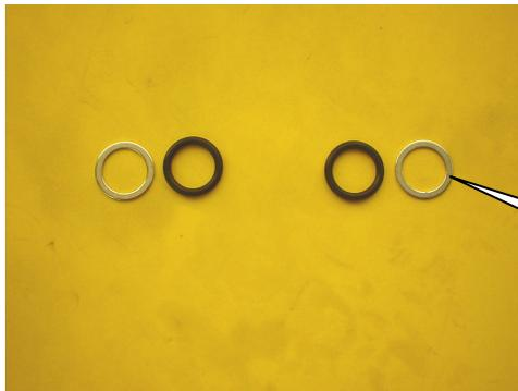
**3;** this image shows the "handle-style" of seal "retainer"...used at **ELITE's** "Body-Mounted Valve"...reuse this when repairing the "seal" here
